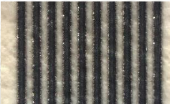
50um wide lines Conductive adhesive on Teslin.
