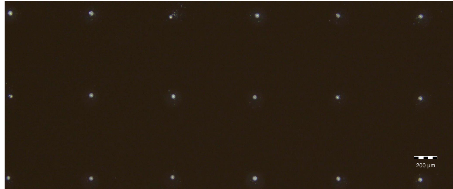
40 \mu\text{m} dots of solder paste
